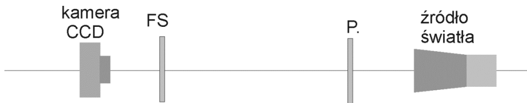
Fig. 5. Measurement of the polarisation characteristics of a light source.
