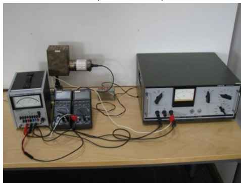
Fig.1. Diagram of electric circuit used in the experiment. (A – ammeter, S – lens, \mu A – microammeter, V – voltmeter, F – interference filter, Z – bulb, D – semiconductor diode)
